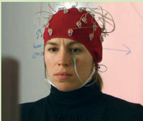
Electroencephalography (EEG) is a noninvasive method for measuring brain activity based on electrical recordings at the scalp.
